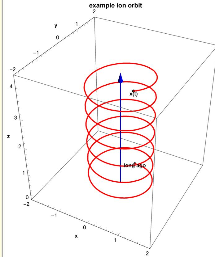
The plasma particle motion is circular in the plane perpendicular to the magnetic field. The velocity parallel to the field lines is constant. Note that  $v_{\perp}$  is also a constant of the motion.
